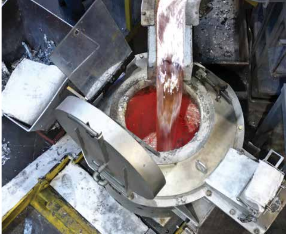
(Transfer of molten aluminum into a transport ladle.) Missouri Smelting Technology employs skilled workers to process and melt aluminum scrap to produce aluminum alloy products such as automotive parts.
